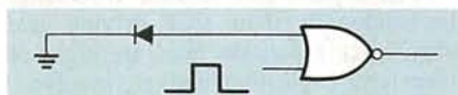
FIG. 7—A DIODE IS USED TO IMITATE a "high" input for an ECL gate.
