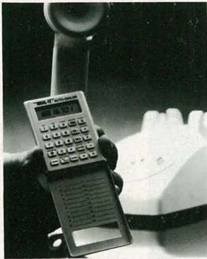
FIG. 11—THIS TINY AUTOMATIC DIALER, the Dial-it from Dictagraph, can store up to 100 numbers.
