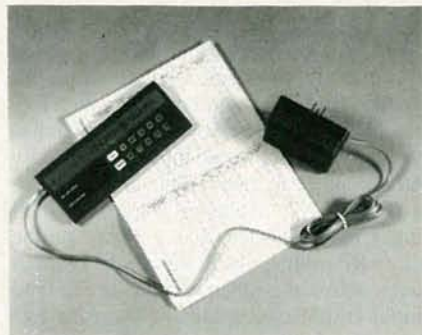
FIG. 14—THE ENERGY$TELLER , sensor module, and log book help keep track of electricity consumption. The system is manufactured by Advanced Micro Products, Inc.
