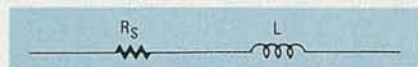
FIG. 2—A REAL INDUCTOR can be represented as an ideal inductor in series with a resistor.
