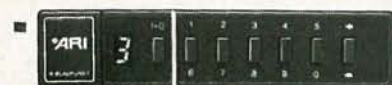
FIG. 10—IN THE ARI SYSTEM, special signals keep a driver informed of traffic reports in his area. The adapter shown here will adapt a Blaupunkt car stereo to receive those ARI signals.
